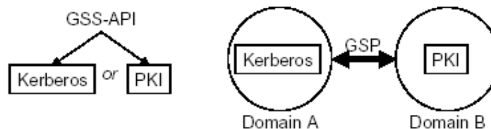
Figure 5: On the left, an API is used to develop applications that can target either Kerberos or PKI security mechanisms. On the right, protocols (the Grid security protocols provided by the Globus Toolkit) are used to enable interoperability between Kerberos and PKI domains.
